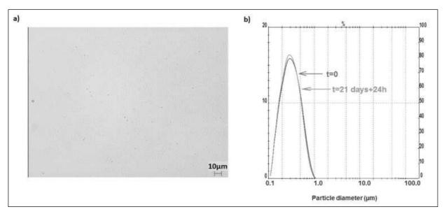
Fig. 1.—Microscopic observation (scale 10  $\mu$ m) at t = 21 days+24h (a) and distribution of oily droplets of TPN admixture 14A (b).
