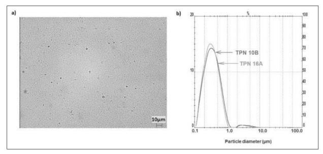
Fig. 2.—Microscopic observation (scale 10  $\mu$ m)(a) and distribution of oily droplets of TPN admixtures at t = 21 days+24h (b).
